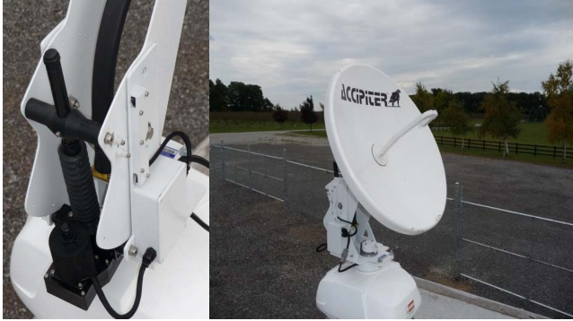
Figure 3: Dish antenna with electro-mechanical vertical scan control, integrated with COTS marine radar. Provides 360 deg azimuth scanning with elevation angle set under software control.
